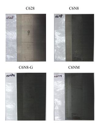
**Fig.4.** Scotch tape test results on the annealed ES (50CS1300) with the investigated coatings. For each photo, the left is the peeled Scotch tape and the right is the annealed sample with tape peeled.
