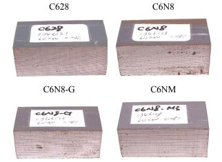
**Fig.6.** The appearance of S-162N punch oil-covered cutting edges of ES (50CS1300, substrate sulfur content = 0.008%) with different coatings after 109 days atmosphere exposure (the photo for Day 109 in Figure 5(d)).
