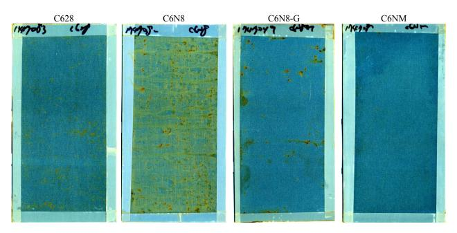
Fig.2. 5Hrs salt spray test results for ES (50CS1300) with different coatings: C628, C6N8, C6N8-G, and C6NM.
