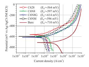
**Fig.3.** Polarization curves for ES (50CS1300) with different coatings (C628, C6N8, C6N8-G, C6NM) and as bare substrate.
