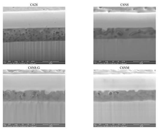
**Fig.1.** The cross sectional SEM images ( $65000 \times$ ) for ES (50CS1300) with different coatings: C628, C6N8, C6N8-G, and C6NM.
