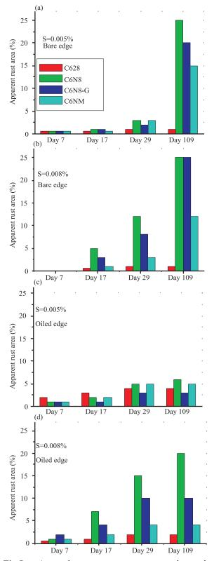
**Fig.5.** Atmosphere exposure test to evaluate the anti-rust capability of the coatings on cutting edges of ES (50CS1300): (a) bare, substrate sulfur content = 0.005%, (b) bare, substrate sulfur content = 0.008%, (c) with punch oil, substrate sulfur content = 0.005%, (d) with punch oil, substrate sulfur content = 0.008%.
